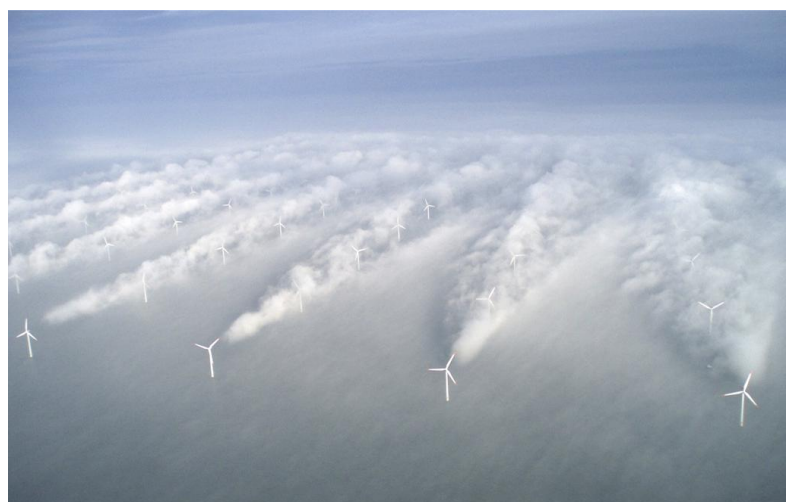
Figure 7: Wakes behind wind turbines at Horns Rev offshore wind park
