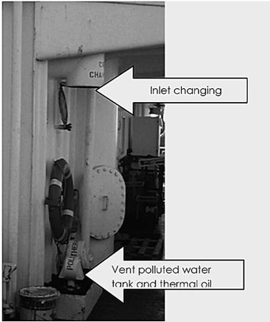
**Figure 6:** Positioning of inlet changing room relative to vent polluted water tank and thermal oil tank.
