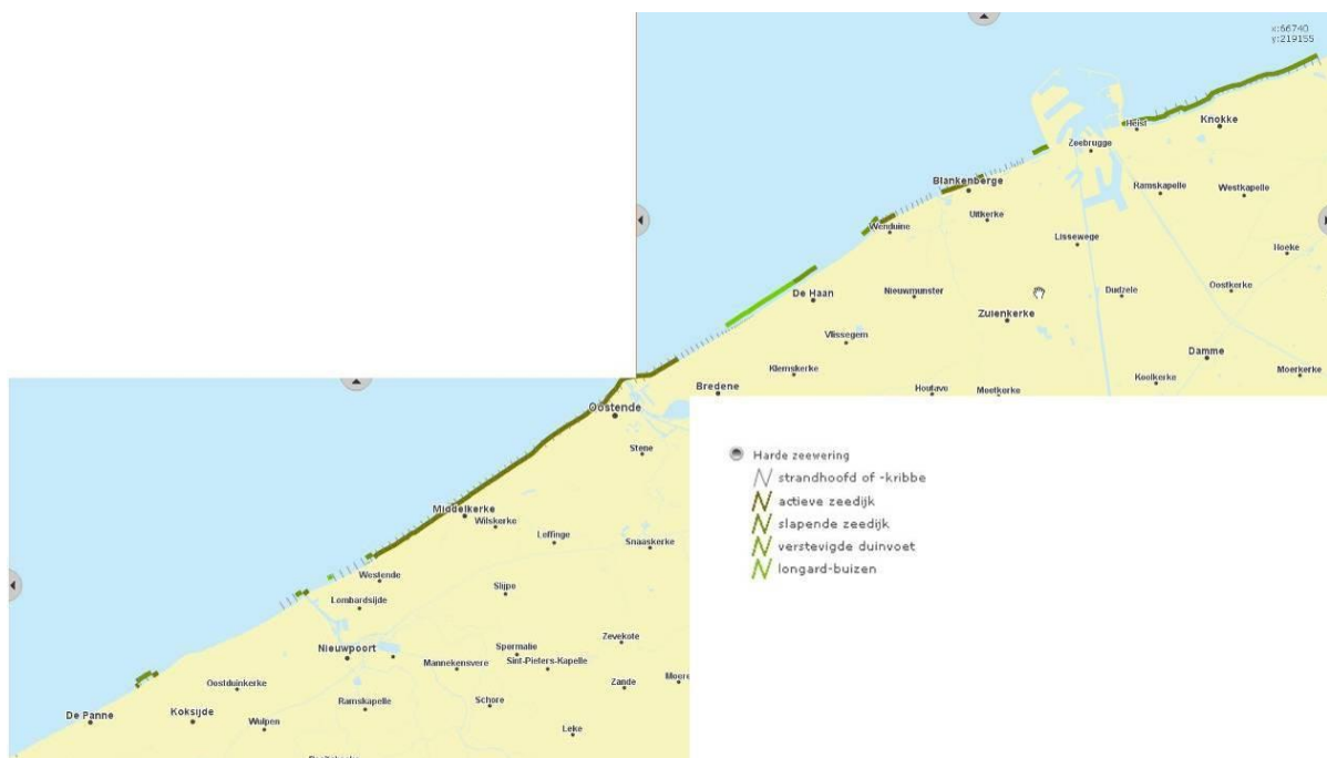
Figure: Hard coastal defence at the Belgian coast [Source: http://www.kustatlas.be/map/?lan=nl&theme_id=5 , consulted on 7/11/2012] xvii .
