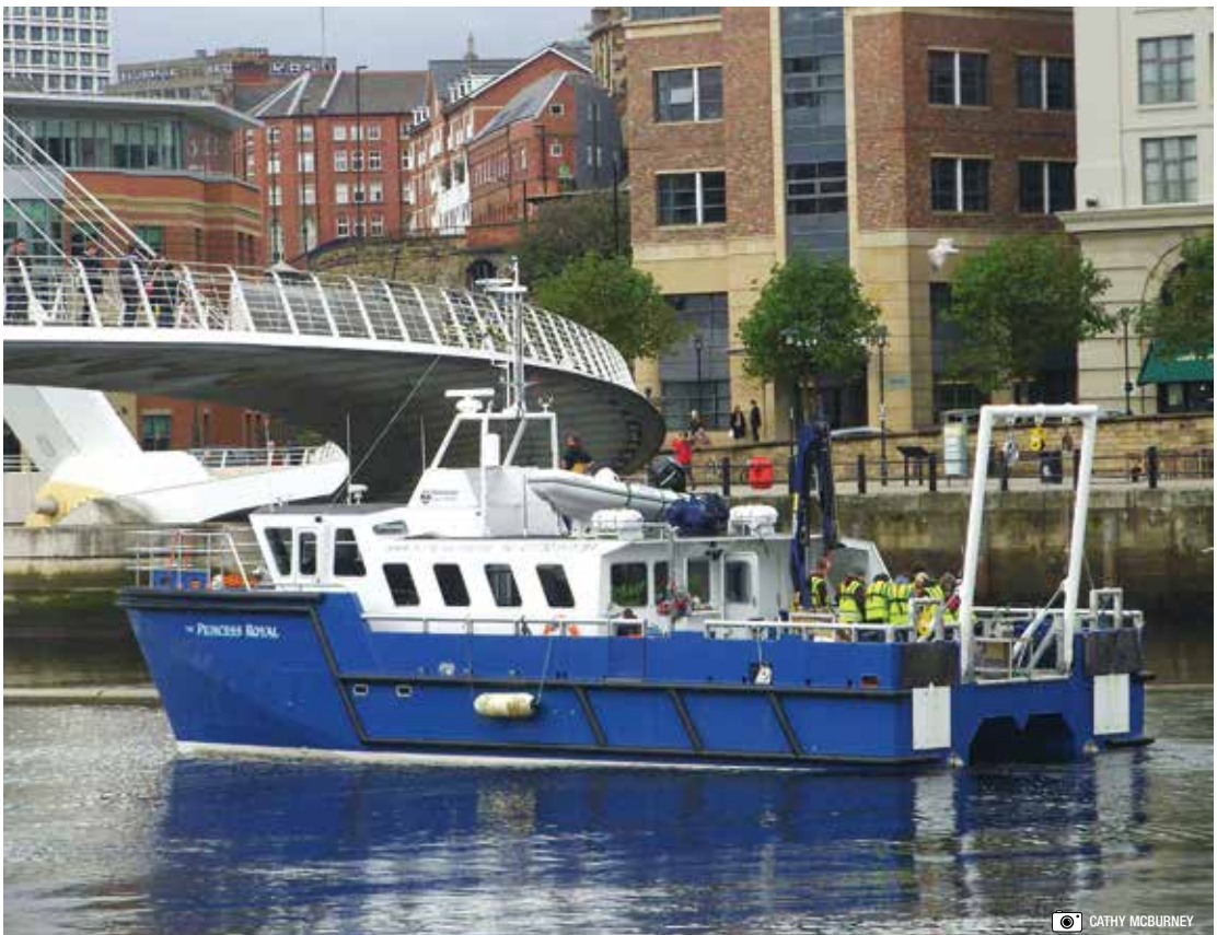
The RV Princess Royal is a coastal research catamaran owned by Newcastle University (United Kingdom) and is more power efficient than conventional designs. The hull, rudder and propellers have been fully optimized to keep fuel consumption and thus engine exhausts low while enhancing sea keeping and speed potential.
