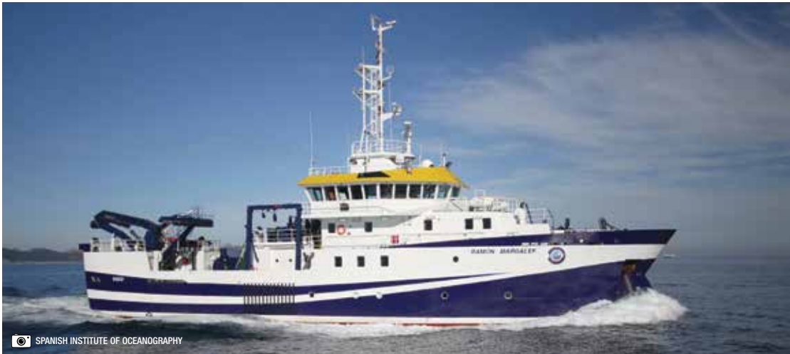
The RV Ramón Margalef is the new research vessel of the Spanish Institute of Oceanography. The vessel uses biocide-free silicon hull paints, ozone treatment of ballast water, and bio-hydraulic oils; sails in a silent mode; houses a power management system; and carries a clean ship notation.
