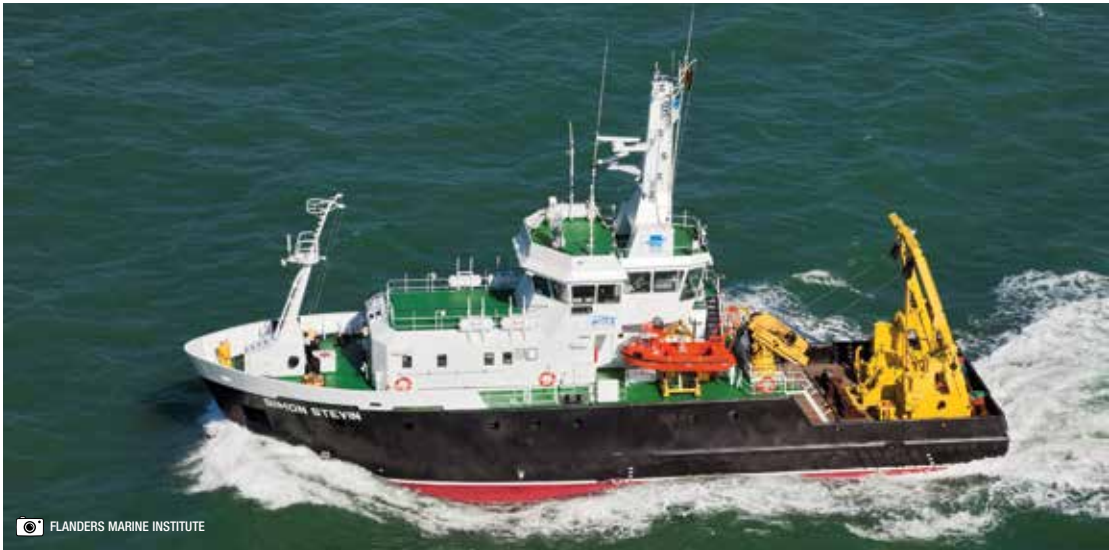
The RV Simon Stevin is the new build coastal multi-purpose research ship of the Flanders Marine Institute, Belgium. The ship carries an active anti-fouling system and a silicone based hull paint, uses waste heat recuperation, has a low noise profile, burns low sulphur fuel, and carries the ISO14001 accreditation.
