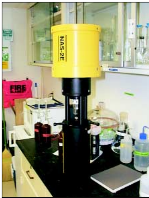
In situ nutrient analysers will increasingly be used for monitoring nutrient loading. Upon laboratory calibration, they can be deployed for periods of weeks to months. Photo by M. Trice.
