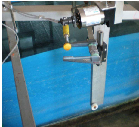
Figure 11. Displacement meter for surge movements: it is a rheometer with a wire mounted vertically and redirected in the horizontal direction by a lower wheel.
