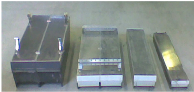
Fig. 3. Four structures tested in the wave flume.
