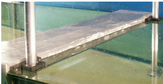
Fig. 9. Detail of pile connection. Physical model test
