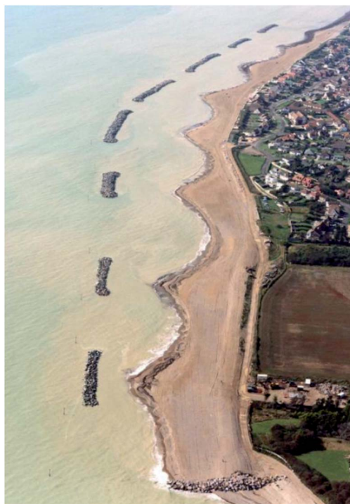
Fig. 3 The Elmer coastal defence scheme in the UK comprises 8 offshore breakwaters positioned parallel to the shore. This image provides a clear illustration of how a network of artificial structures can provide stepping-stones facilitating the spread of marine species, especially those with poor dispersal capability.
