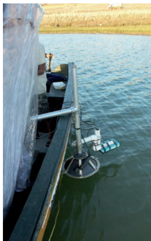
▲ © MMRG. A Knudsen 320 BP Echo-sounder and external receiver, modified by Prof. Lloyd Huff (Center for Coastal Ocean and Mapping, University of New Hampshire), prior to submersion during the Morocco Maritime Survey, Morocco.
