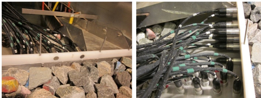
Fig. 4. (Left) Front view of attachable sections with pressure transducers for raising the unprotected crown wall height. (Right) Pressure transducers on the rear side of the wall.
