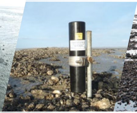
^ Sensor used to measure wave attenuation above an oyster bed Picture: Jim Van Belzen
