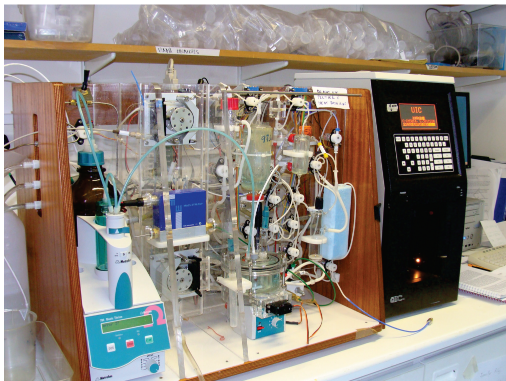
Figure 4.1. VINDTA 3C system for semi-automated measurement of DIC and TA. Photo: Pamela Walsham.
