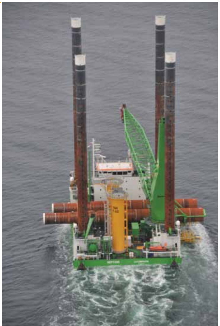
Vessel on its way to the Nortwind site on the Lodewijk-bank with two monopiles and two transition pieces.
