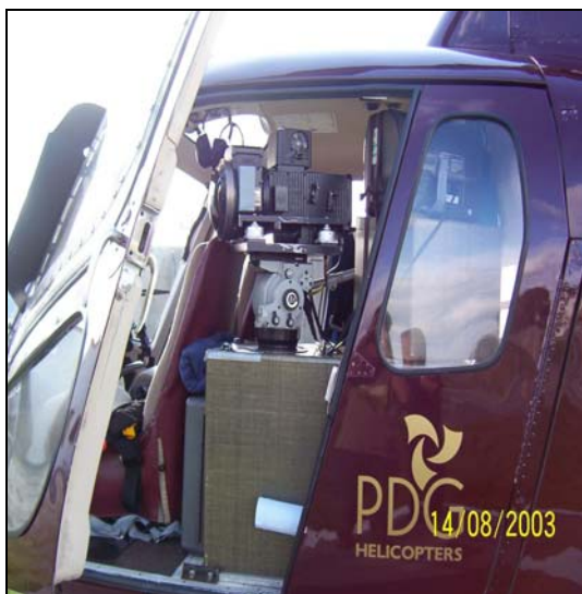
Plate 2. Position of thermal-imager in helicopter.
