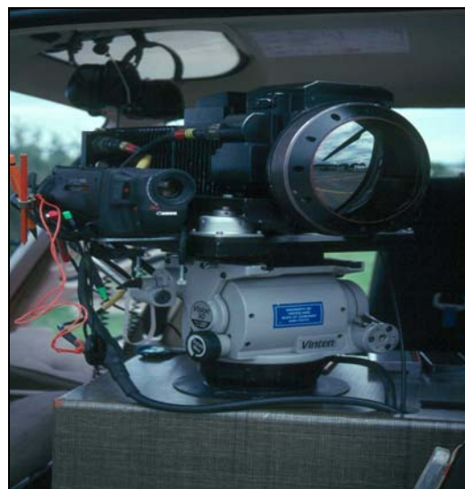
Plate 3. Thermal-imager mounted on pan & tilt head.
