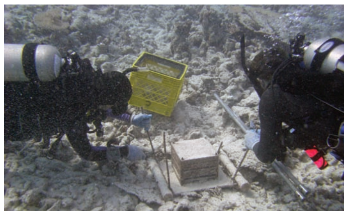
Autonomous Reef Monitoring Structures, layered plastic structures likened to empty dollhouses, are retrieved from French Frigate Shoals. Photo: U.S. National Oceanic and Atmospheric Administration, Pacific Island Fisheries Science Center, Northwestern Hawaiian Islands Marine National Monument.
