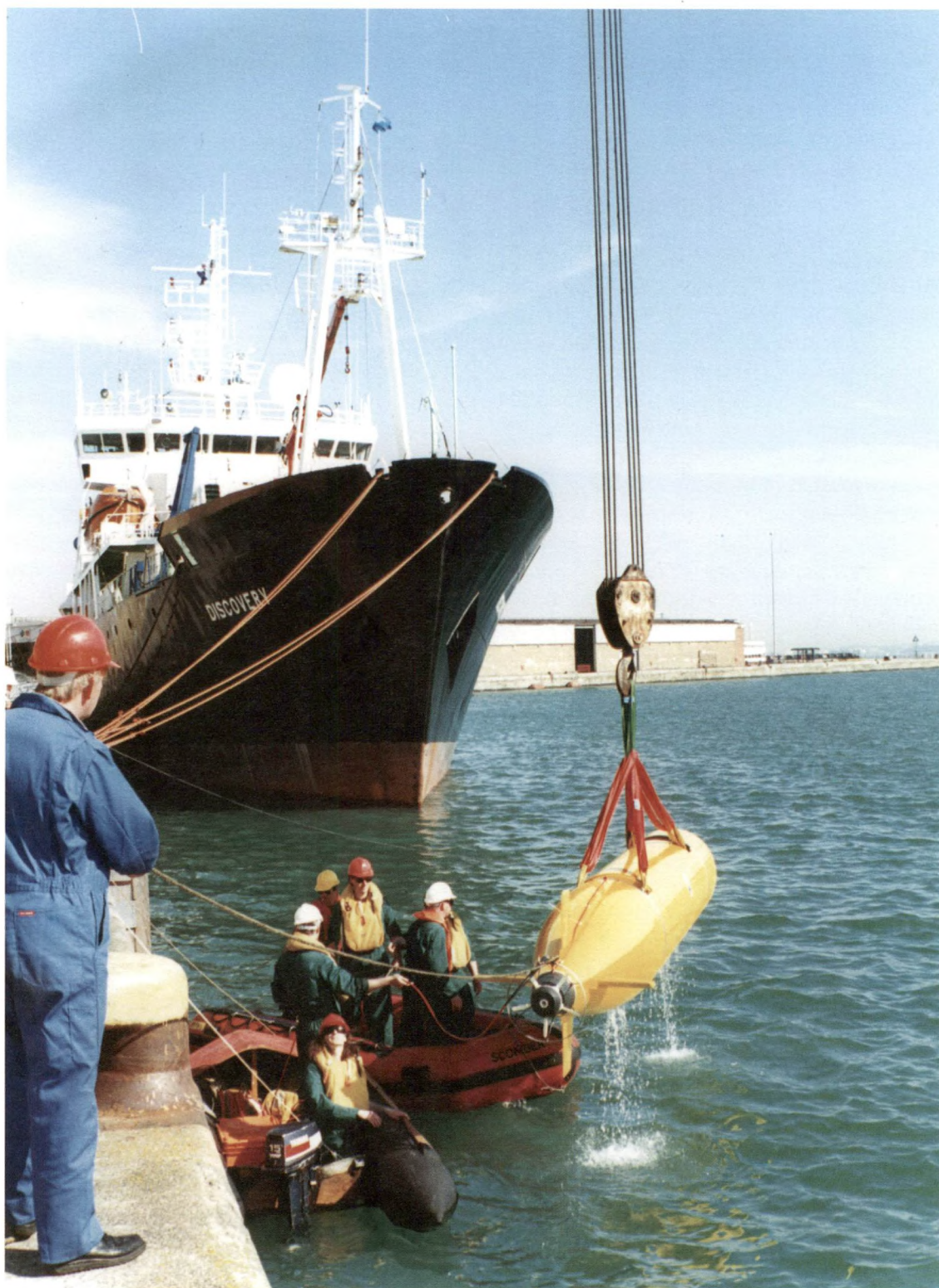
The Autosub-1 is an autonomous underwater vehicle which can travel hundreds of km making measurements of the state of ocean water. The demonstrator vehicle undergoing sea trials in this picture was part funded through a MAST project. Development work was carried out by NERC and IFREMER. Source: SOC
