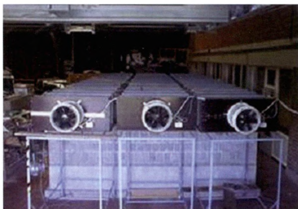
Figure 4. Test installation for ammonia emission measurements
