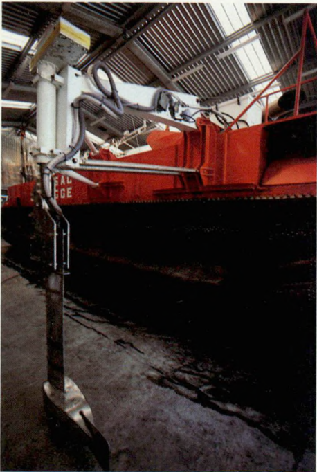
fig. 7 : hydraulic retractable arms with sword and fish.
