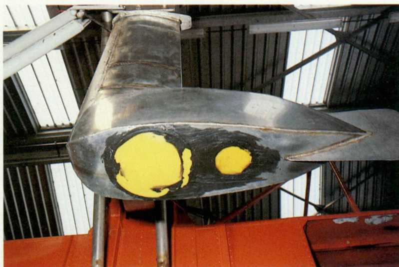
fig. 16 : bottom view of a fish with two acoustic transducers.
