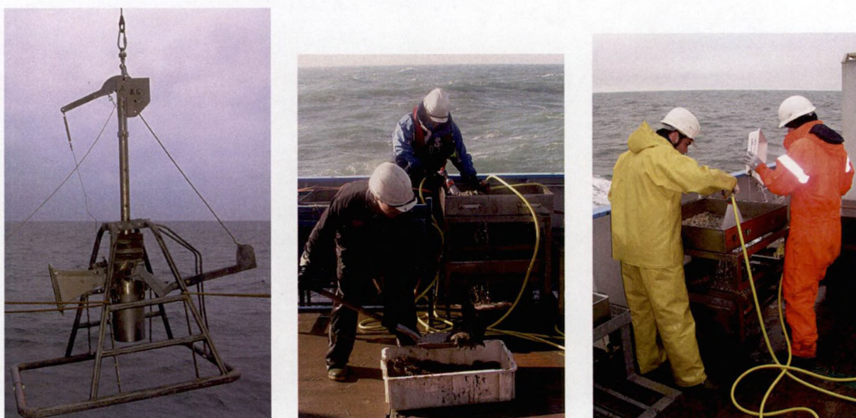
Figure 5. Reineck boxcorer for sampling infauna. Sampling size 0.07 \text{ m}^2 to a depth of 40 cm. Samples are washed over 1 mm sieves.
