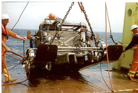
Figure 3. Triple-D dredge for sampling larger sized and lower abundant infauna and epifauna. Sampling area: a strip 80 m long and 20 cm wide ( 16 \text{ m}^2 ) to a depth of 18 cm. Meshsize of the netting 1.4 cm stretched (Bergman and van Santbrink, 1994).
