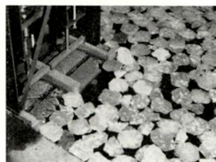
Fig. 6. Discharge of ice floes using auxiliary outlets. Development of ice bridges.
