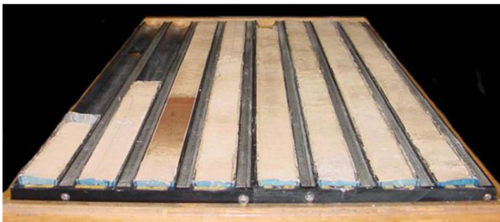
Figure 4.2. Atlantic Ocean deep-sea core from the Integrated Ocean Drilling Program. Note the brown section of the core, which represents the dissolution of deep-sea carbonate at the Paleocene-Eocene boundary. This could represent a lack of calcifiers during that time period or the dissolution of dead shells. Source: James Zachos.
