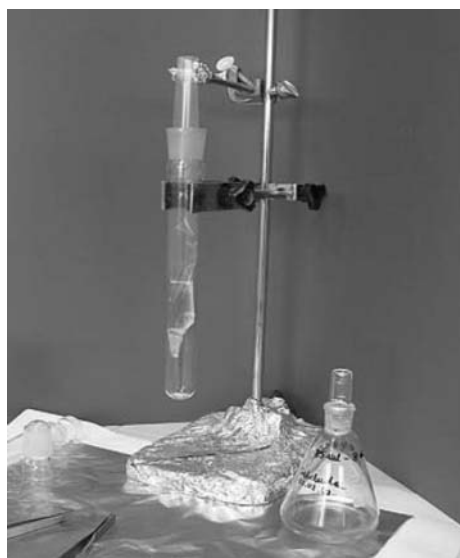
Fig. 2. Membrane filled with fat extract
