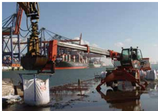
Fig. 2.22. The Manitou, a crane with a long hydraulic jib, moved the bulk bags to the back of the pontoon moored alongside the Triton .
