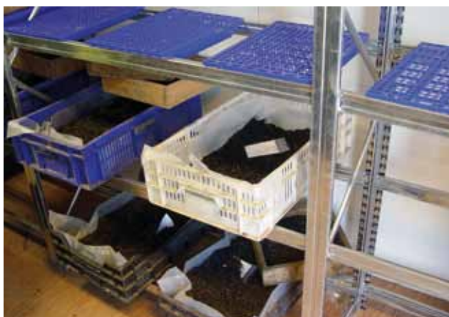
Fig. 2.28. The 10mm and 2mm-sieve residues were dried on site in a specially equipped container.
