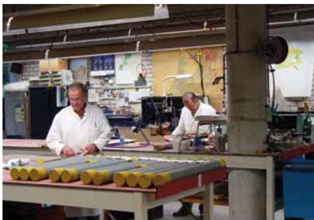
Fig. 2.9. At TNO Geological Survey of the Netherlands' sediment registration laboratory in Utrecht, the coring tubes were cut open and the cores prepared for further analysis.
