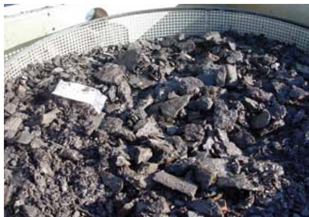
Fig. 2.26. Detail of a soil sample on one of the 'Lutter' sieves. The lumps are some of the many peat fragments that were left on the mesh after sieving each batch.
