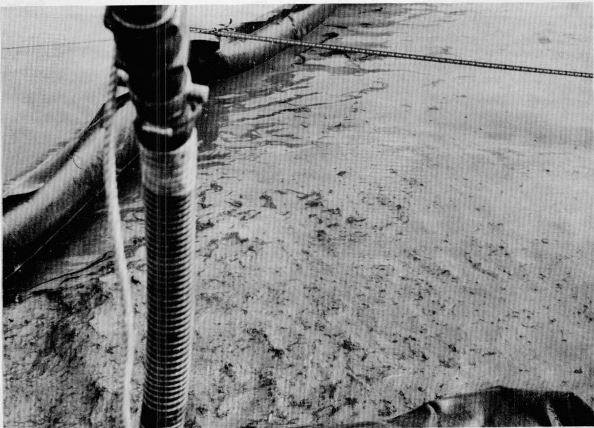
Figure 2 Application of amine-treated sand on to oil held in a boom.
