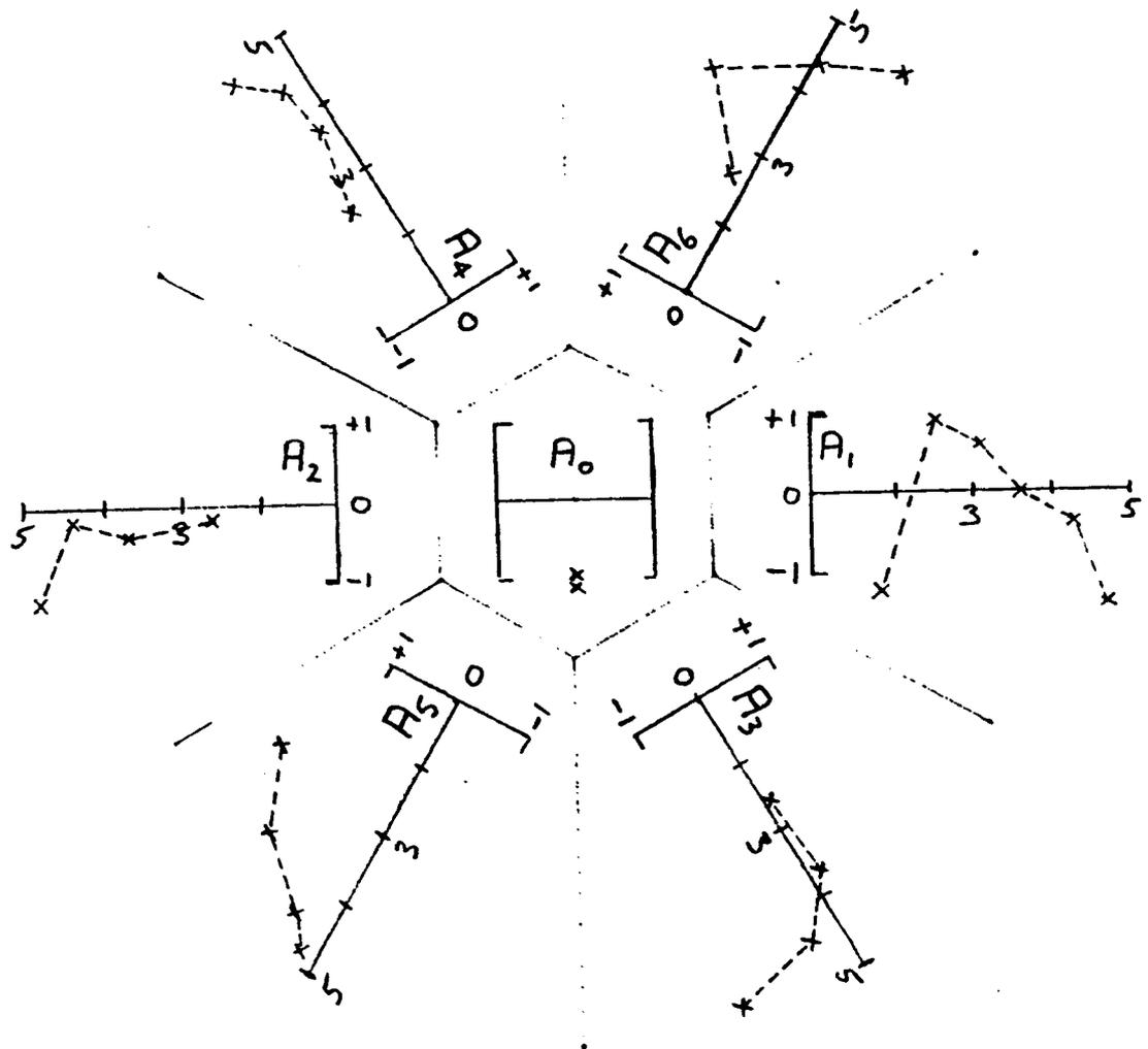
Figure 3. Indicated TS as a function of the target position in the beam. Second calibration. Measurements are shown by sub-area. Radial axes - target direction relative to the acoustic axis, degrees; azimuthal axes - indicated TS, dB relative to the mean TS from Table II.
