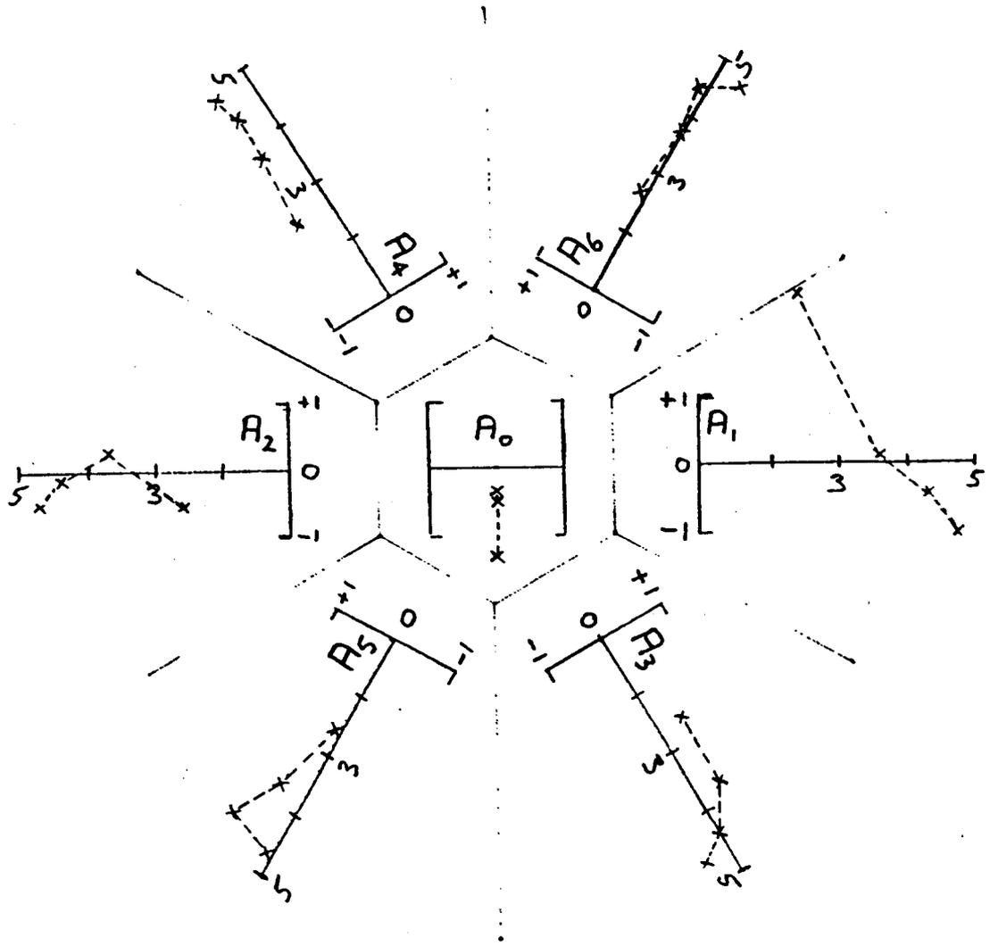
Figure 2. Indicated TS as a function of the target position in the beam. Measurements from the first calibration are shown by sub-area. Radial axes - target direction relative to the acoustic axis, degrees; azimuthal axes - indicated TS, dB relative to the mean TS from Table II.
