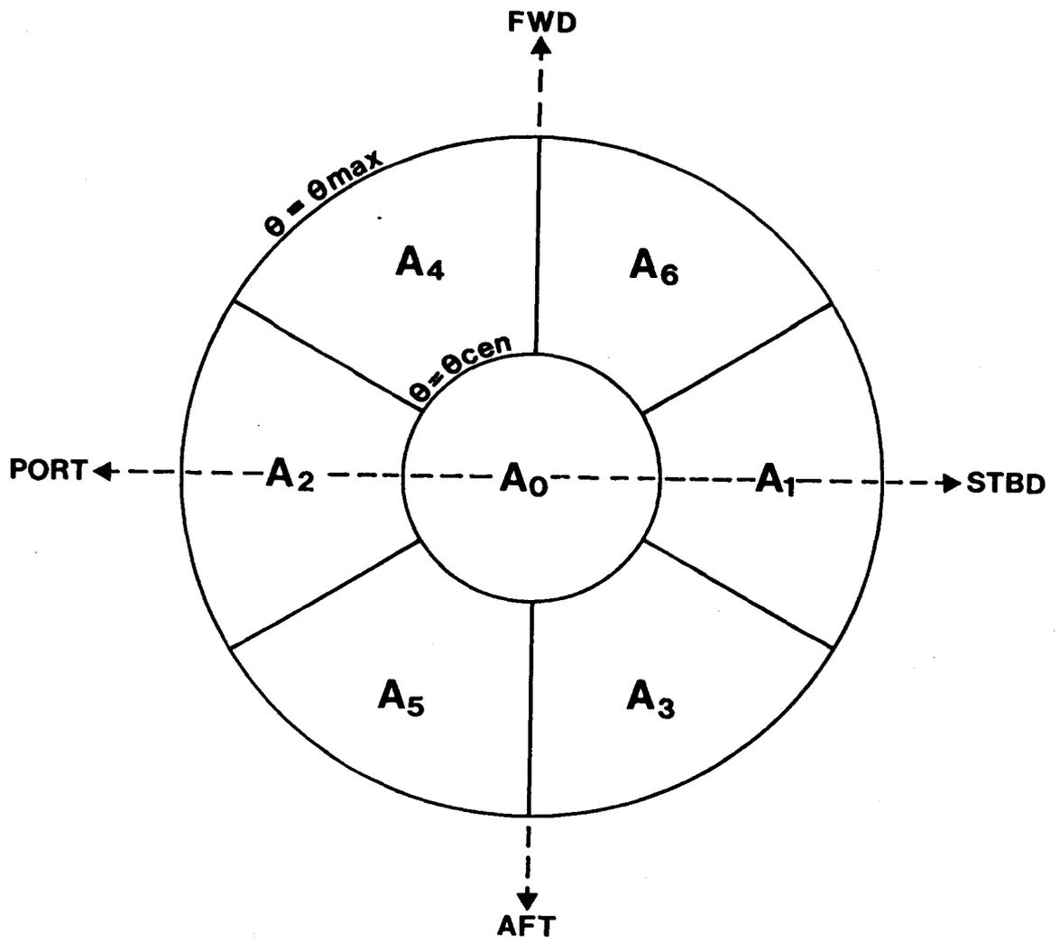
fig 1. Division of the beam cross-section into seven equal sub-areas
