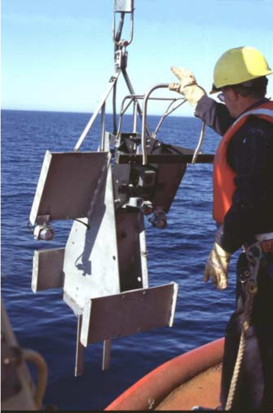
Figure 1. Photograph of the Towcam fish (1999 version) being deployed off the stern of the C.C.G.S. Hudson .
