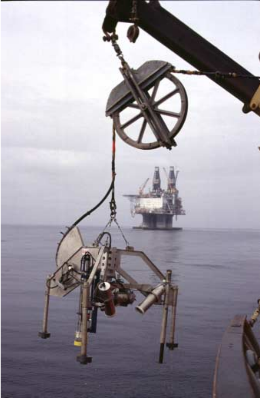
Figure 2. Photograph of Campod being deployed from the C.C.G.S. Hudson near the Hibernia oil platform on the Grand Banks.
