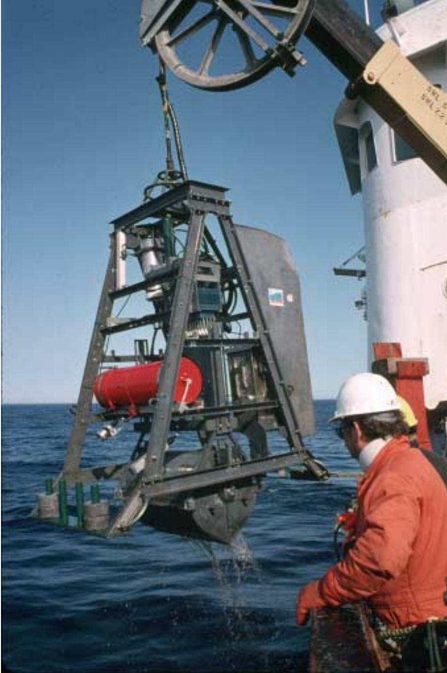
Figure 3. Photograph of the videograb (equipped with DRUMS™) being recovered by the C.C.G.S. Hudson .
