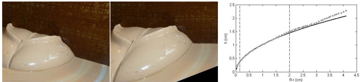
Fig. 8. Photo of the slump test used to measure the final profile, original (left) and after rectification (right). On the far right a digitalized profile (o) and its least square fit (solid line) is shown over the selected zone (between the vertical dashed lines).
