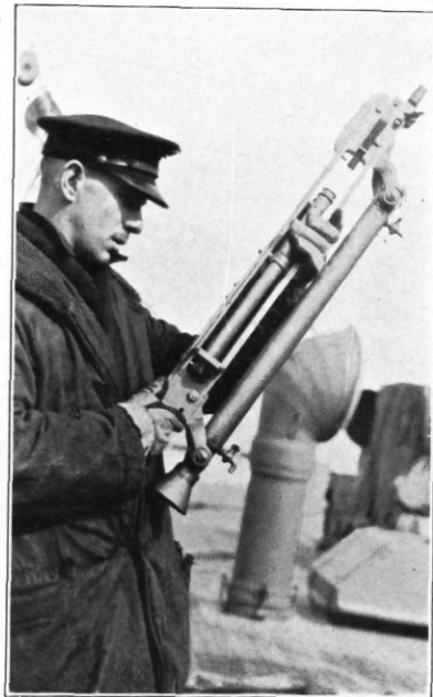
PLATE IX.—Reading the reversing thermometers in a Greene-Bigelow water bottle that has been tripped on the wire at a known depth and then hoisted up and taken aboard. The cylinder fitted with two pet cocks contains over a quart of sea water from the level at which the bottle was tripped
