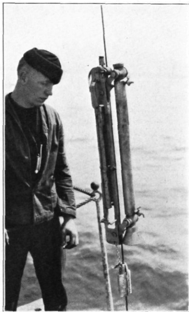
PLATE VIII.—A Greene-Bigelow water bottle clamped to the sounding wire. Seven such metal bottles are clamped on at different points and lowered into the sea at each oceanographic station. The upper bottle is tripped when a messenger is slid down the wire. In tripping, a messenger is released from the bottom of the bottle to slide down to the next one in the series, and so on
