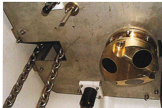
Current sensors at Texel ferry monitoring platform
