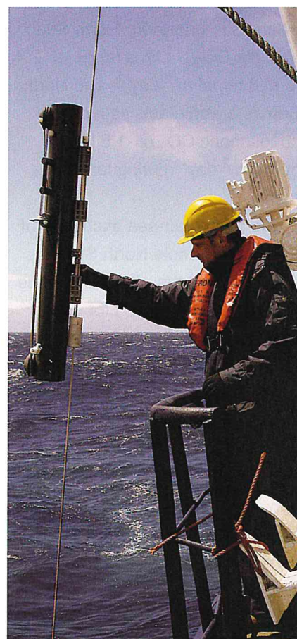
Patrick Laan collects "iron-free" water with GoFlo bottle attached to kevlar cable in the Southern Ocean.
