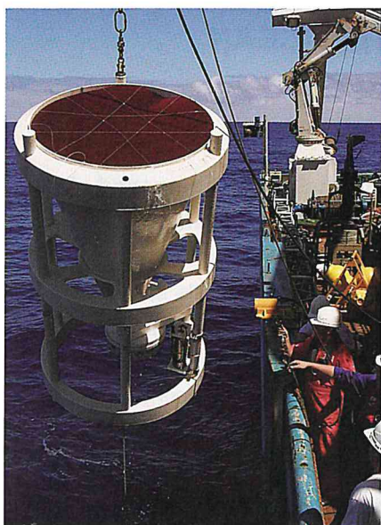
A large sediment trap is recovered from 2700 m depth after collecting samples and sensor data for half a year in the Southeastern Atlantic.
