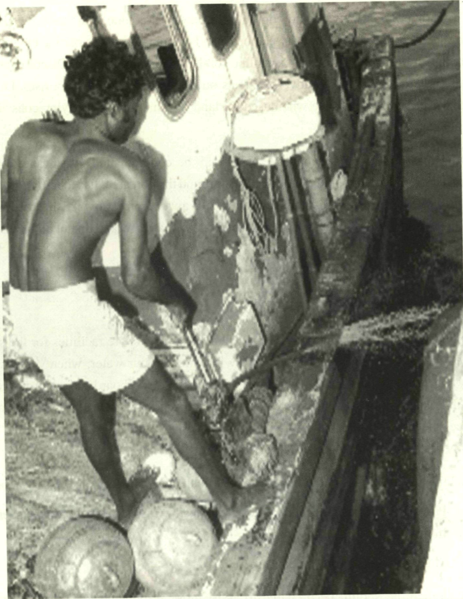
Figure 33 A TYPICAL SCENE INSIDE A FISHING HARBOUR - BILGE WATER BEING PUMPED OVERBOARD
