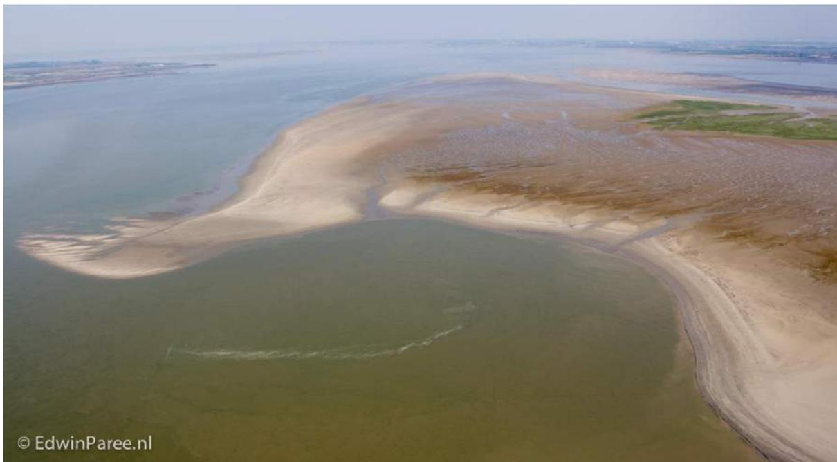
*Figure 1 Aerial view of the gap created by the 22 July 2014 flow slide on the tidal flat of Walsoorden, Zuidergat and in the distance Perkpolder (E. Paree, September 2014).*
