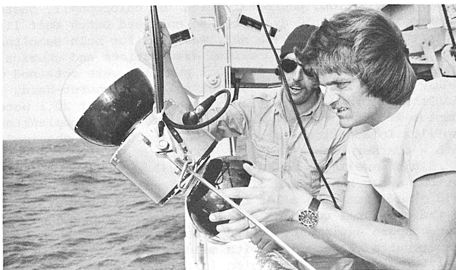
NECTAR (2.09.3). Plankton recorder, macro-plankton catch and inspection of the spectral irradiance meter.
