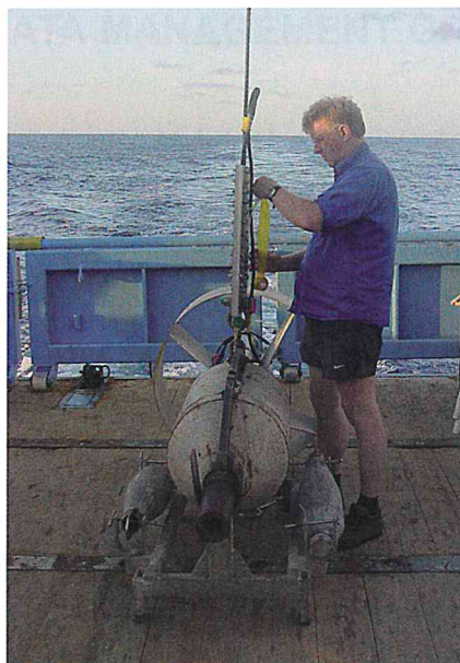
LOCO/IW preparing the towed ADCP for testing.
