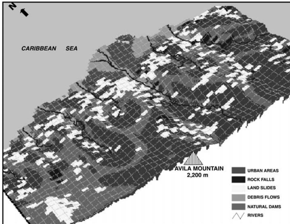
Figure 3. Model sustainability output combining the slope model and the coverages: hydrology, infrastructure, and land mass movements. The land masses considered were: rock falls, landslides, debris flows and natural dams.
