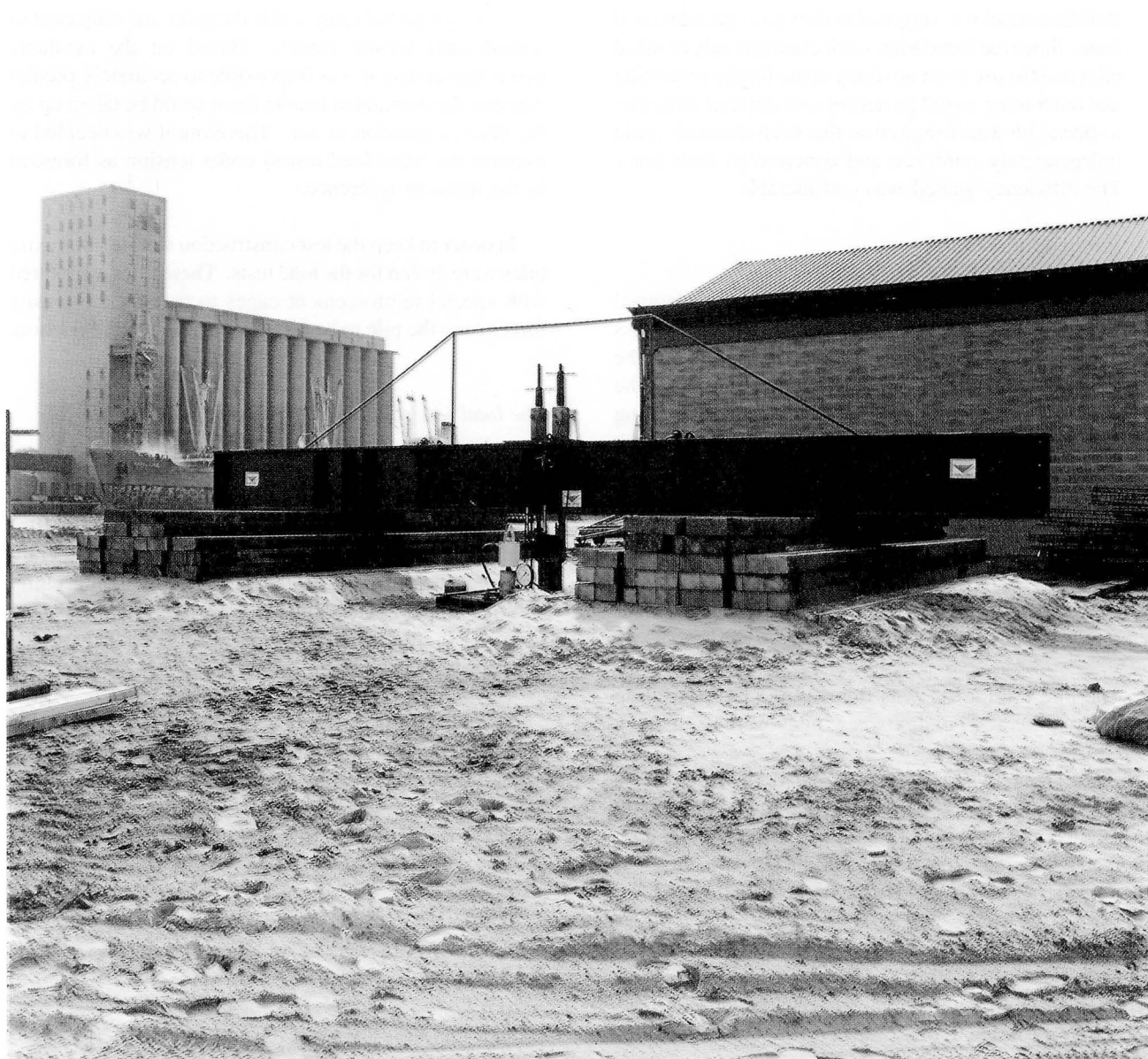
Fig. 52 — Pull load test — Test set-up.
