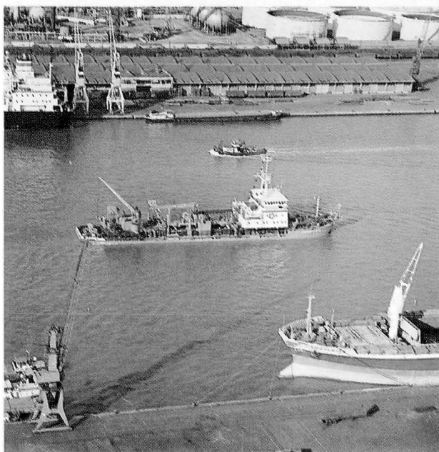
Fig. 66 — Towed hopper suction-dredger "Krankeloon".
