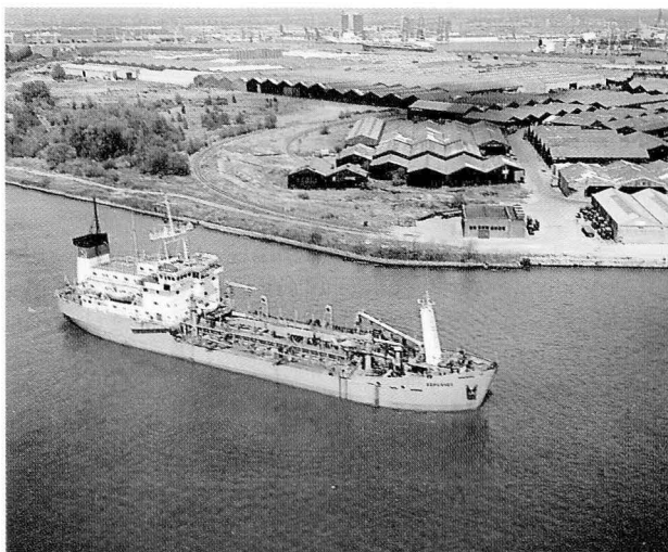
Fig. 68 — Towed hopper suction dredger "Khersones".
