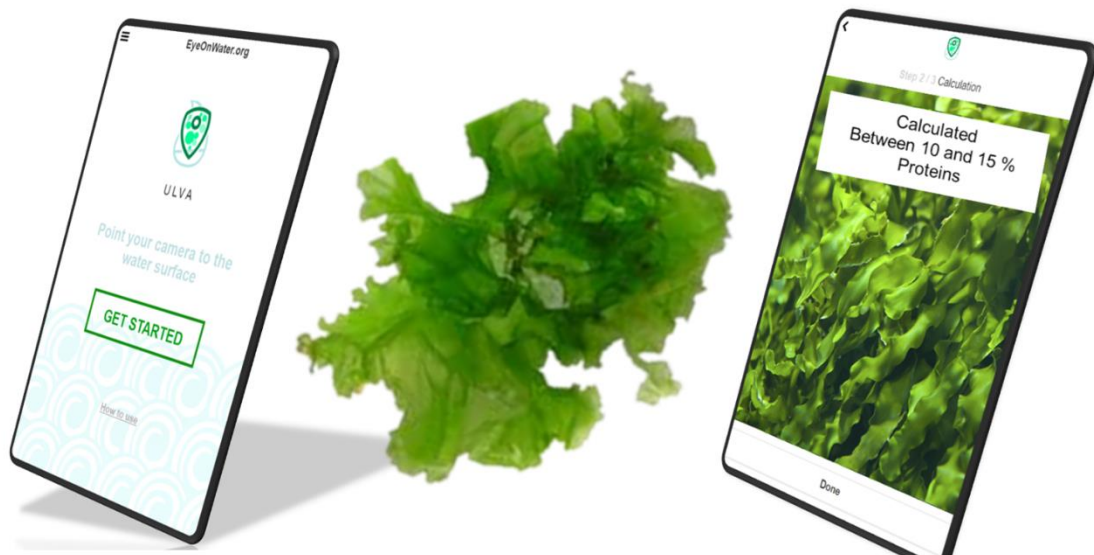
Figure 1-6. The smartphone application ‘EyeOnUlva’ for Android and IOS systems ( www.eyeonwater.org/ulva ) records the frond colour of the green seaweed Ulva lactuca and provides a fast quantification of its total dissolvable protein concentration in % dry weight. The data can be send to a data base, which is part of the CITCLOPS project ( www.citclops.eu ).
