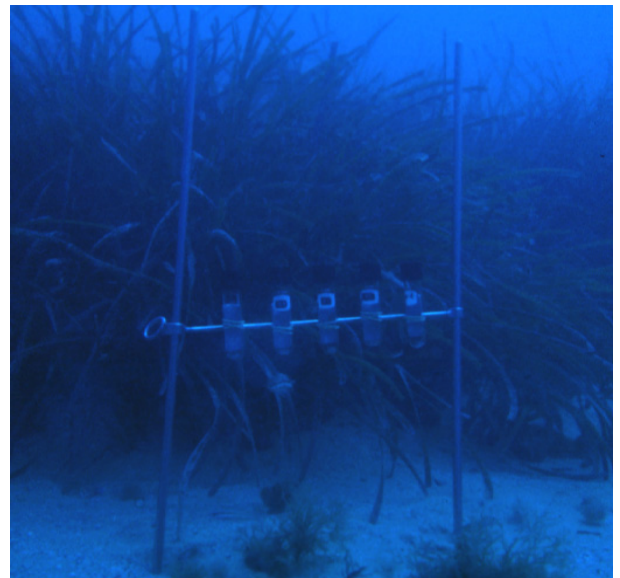
Figure 10.1. Benthic sediment trap deployed within a Posidonia oceanica bed. Photo: Carlos M. Duarte.
