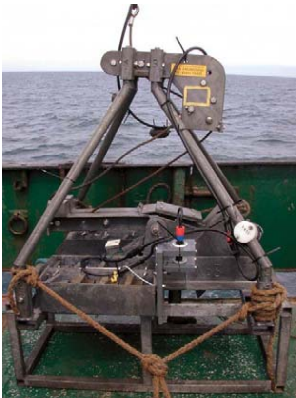
Figure 3.1. A 0.1m 2 Hamon grab with attached video camera supported on an open frame to facilitate retrieval of the sample into a moveable container following controlled release from the grab bucket
