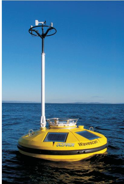
**Figure 4.1:** The Wavescan heave/pitch/roll data buoy,  $\text{\O}2.8\text{ m}$  (*Photograph used by permission*).
