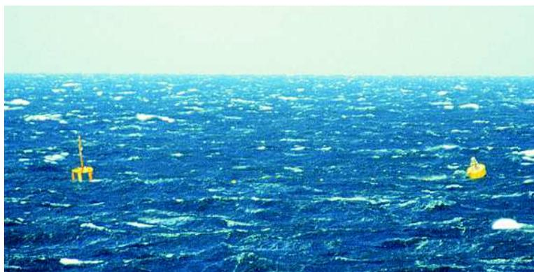
**Figure 4.10:** ASIS and tether buoys at sea during a Mistral event (FETCH experiment, Hauser *et al.*, 2003). The two buoys are connected by a 60 m floating tether, with the latter buoy moored to the bottom.
