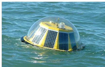
**Figure 4.4:** The TRIAXYS directional wave buoy. (*Photograph used by permission*).
