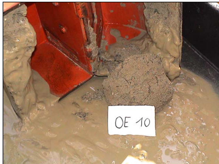
Figure 2.2: Van Veen grab sample of recent mud (1 cm) on top of sand, R/V Belgica campaign 2003/04. (old dumping place Oostende)
