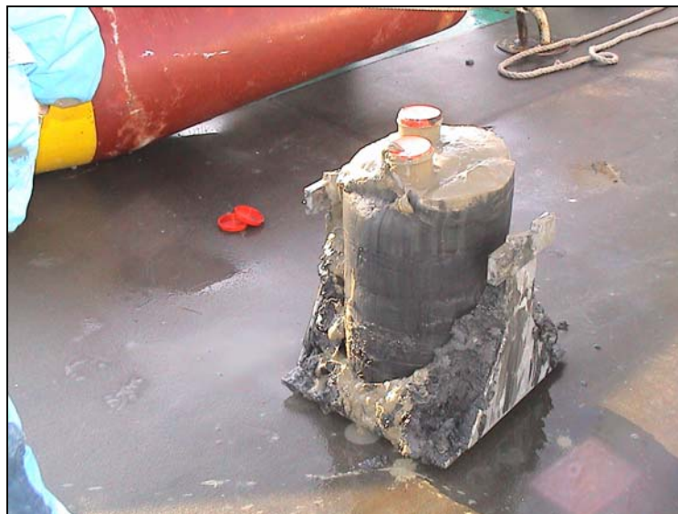
Figure 2.3: Box core (completely filled, 50 cm) of very soft mud, which is gradually more compacted underneath and covered by a recent layer of 7-8 cm mud, R/V Belgica campaign 2003/04 (old dumping place Oostende)
