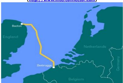
Figure I.2.1b: The pipeline Interconnector in the North Sea (http://www.interconnector.com)
