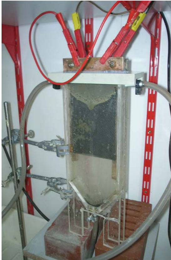
Figure 6.4. View on the electrolysis cell. Gas formation at the electrodes is clear.
