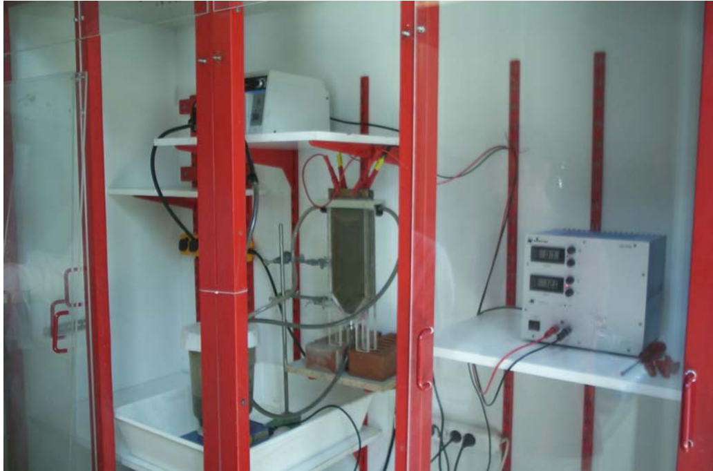
Figure 6.2. Overview of the lab scale set-up at TU Harburg: middle: electrolysis cell, right: current rectifier; left below: reaction tank.
