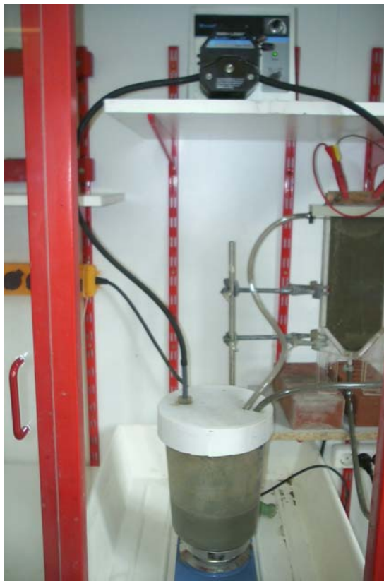
Figure 6.3. Detail of the laboratory set-up: below: sediment buffer, right: electrolysis cell, top: pump.
