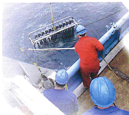
The Titan CTD and water sampler is made of titanium and has been designed and constructed in a close cooperation between the departments of Marine Biology and Marine Technology. It is used to study the influence of iron on plankton growth in the open oceans.
