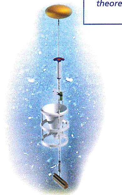
Scheme of a mooring with, from bottom to top: anchor weight, acoustic release mechanism, sediment trap, current velocity meter, acoustic Doppler current profiler and a floater to keep the cable in an upright position. Image: Harry de Porto (NIOZ).
