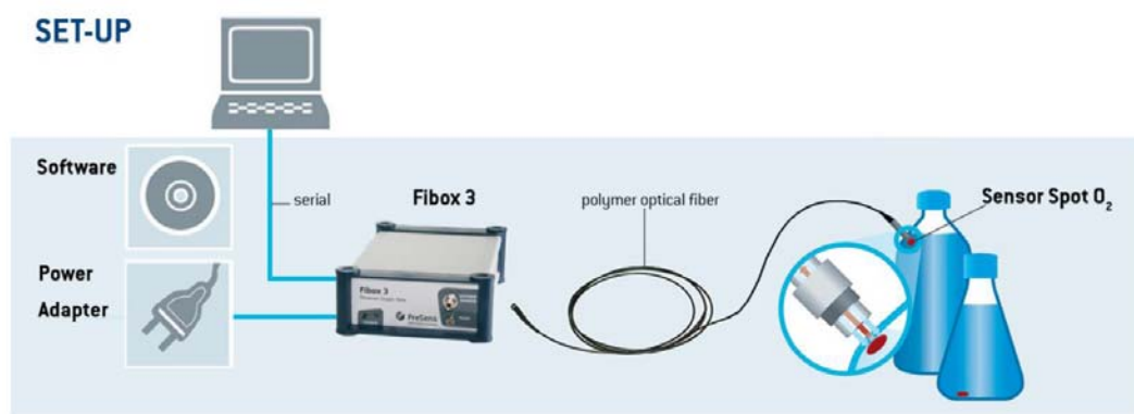
Figure 25. Set-up for measurement with PST3 optodes (PreSens 2016)
