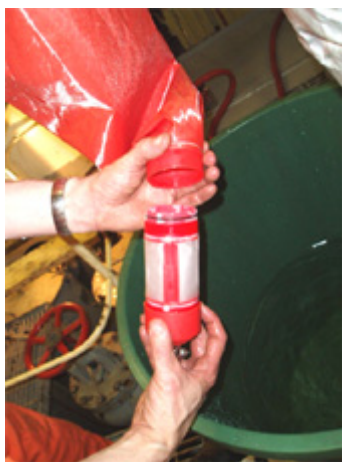
Figure 4. Cod-end may be unscrewed from filtering bag.
