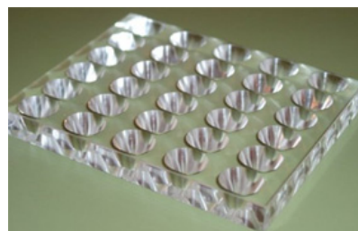
Figure 5. Newly designed zooplankton counting chambers.
