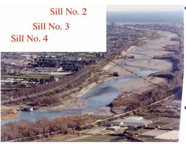
• During the flood event of 5/11/94, sills 2 & 3 collapsed and the flood wave inundated part of the city and airport.
