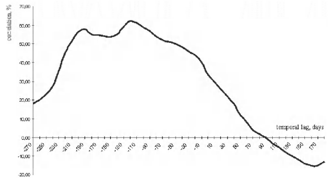
Fig. 4b. Lag-cross correlation function for the temporal coefficients of the second SVD vector: \tau —temporal lag; \tau < 0 : the SST anomalies lag wind anomalies; \tau > 0 : the SST anomalies lead wind anomalies (ENSO 1997–2000).
