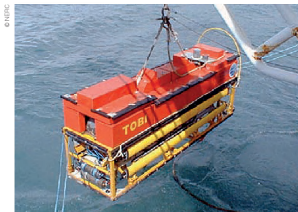
TOBI, a seafloor mapping system
