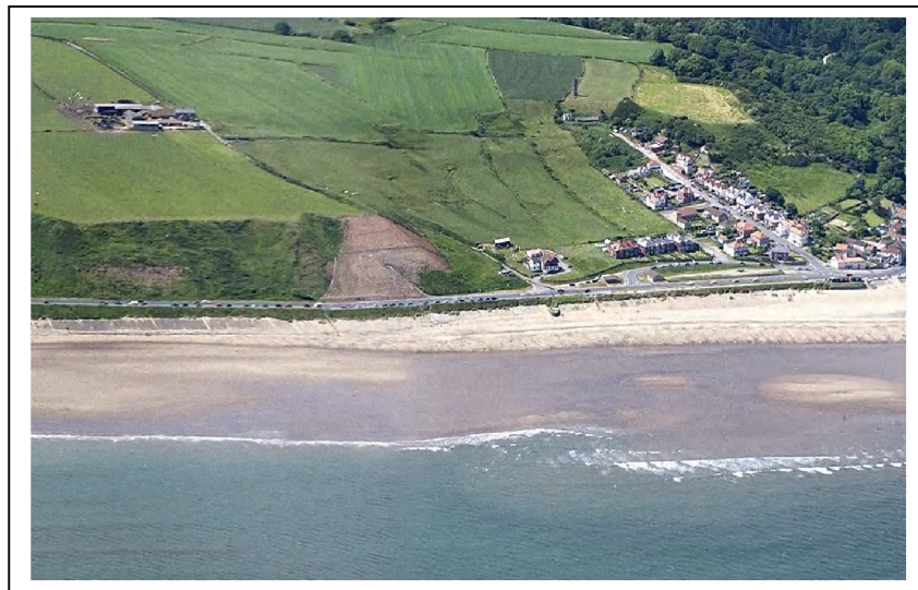
Plate 7.2 Sandsend to Whitby, North Yorkshire, showing recent regrading works following the landslide.
