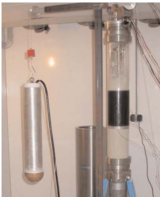
Melting Probe technology of potential use for penetrating layers of ice.
